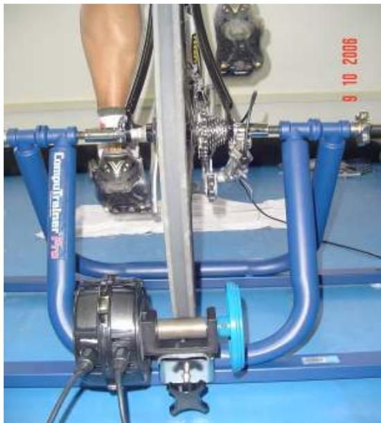
Figura 2: Ciclosimulador *CompuTrainer Professional* modelo 8001 (*RaceMateInc*<sup>®</sup>)
