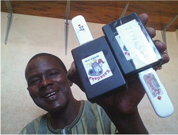
Fig. 7. Adama Tessougué of Radio Sikidolo shows the Kasadaka on which the Foroba Blon voice service now runs with its Bambara language interface [2].
