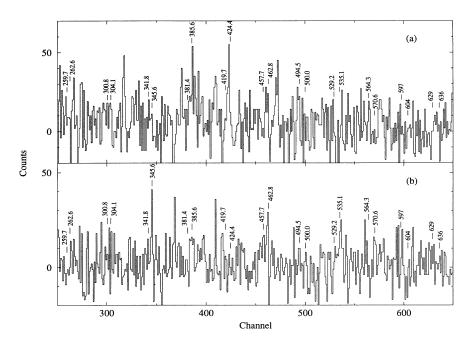
FIG. 2. Coincidence spectra generated for Compton-suppressed Ge spectrometers located at 145.5° by requiring a prompt fold of at least 8 and a coincidence with (a) the 346-keV and (b) the 424-keV transitions, respectively.
