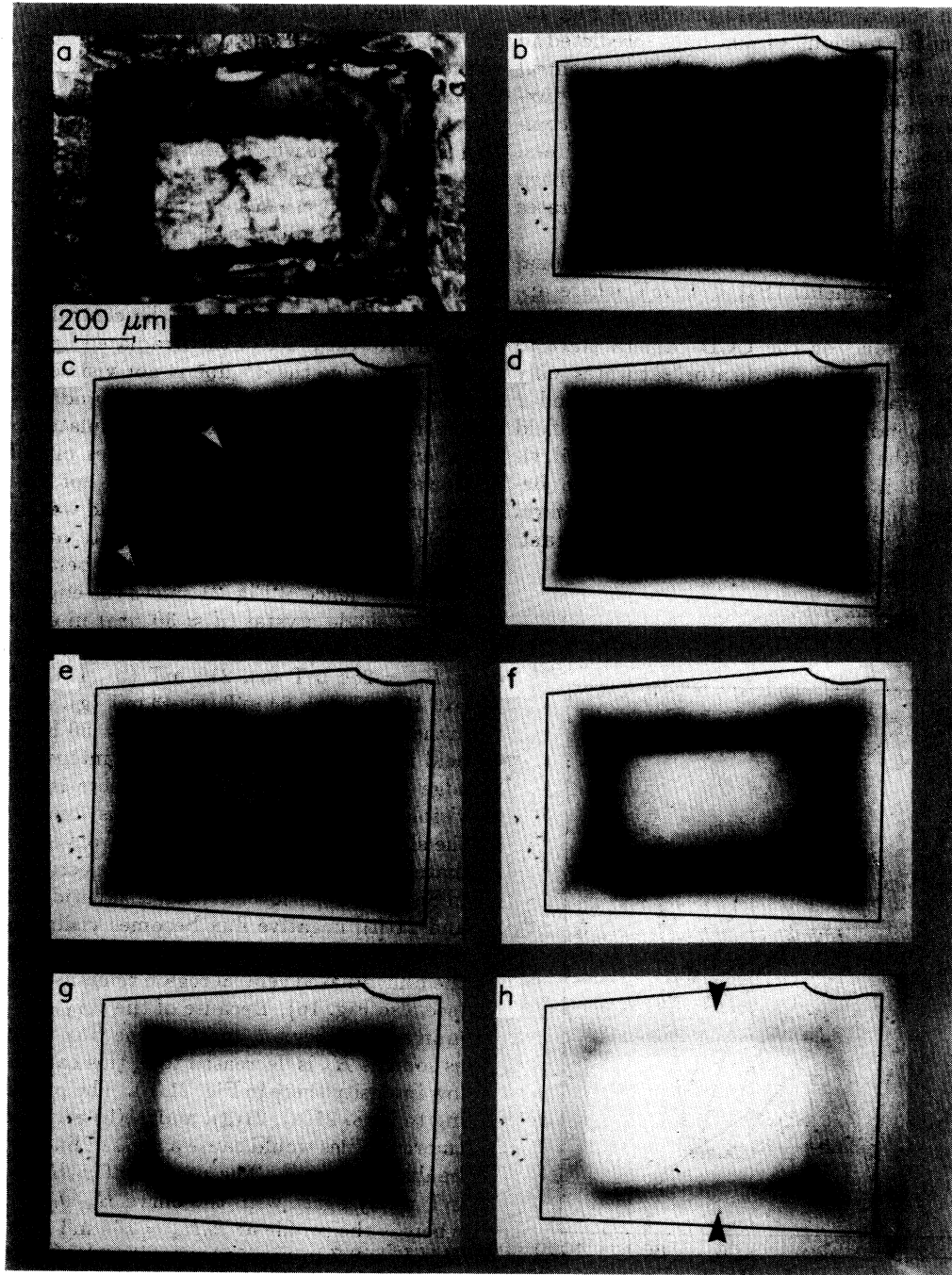
FIG. 19. (a) Shape of the irradiated Bi2212 single crystal. The absorber is visible as bright region in the sample center. (b) Flux distribution at T = 50 K in a transverse magnetic field of \mu_0 H_a = 85 mT. (c) \mu_0 H_a = 107 mT. The flux starts to penetrate the unirradiated part of the sample at the narrowest place of the irradiated belt (white arrow in the lower left corner) and piles up in the sample center as indicated by the other white arrow. (d) \mu_0 H_a = 128 mT. (e) \mu_0 H_a = 149 mT. (f) \mu_0 H_a = 171 mT. (g) \mu_0 H_a = 213 mT. (h) \mu_0 H_a = 277 mT.
