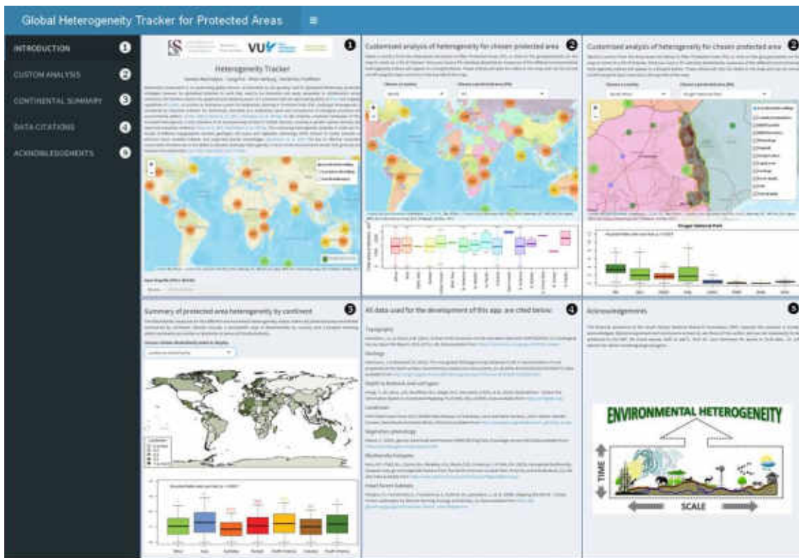
Fig. 6.1: Composite screen view of Heterogeneity Tracker Beta 1.0 structure and functionality, designed using a Shiny framework with embedded Leaflet maps and various summary and graphing functions. Available from https://heterogeneity.shinyapps.io/globalheterogeneity/ .
