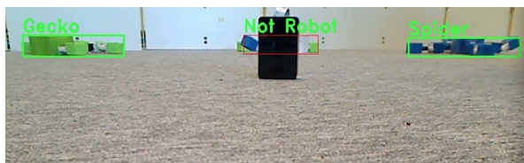
Fig. 5: The recognition for an occlusion situation. The center part of robot ‘Baby’ (middle) is occluded by a black box. The red bounding box is the ROI proposed by FROIS algorithm. The green text above the red bounding box is ‘Not Robot’.
