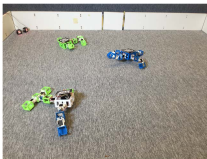
(d) Scheme D: Embodied evolution of controllers and bodies. There is no centralized evolution manager; selection and reproduction are regulated by the robots and their interactions.
