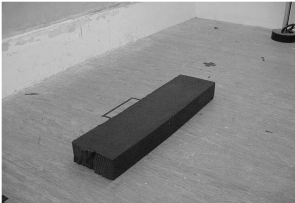
Figure 8.1 - The selected sound absorbing material of thickness 150 mm.
