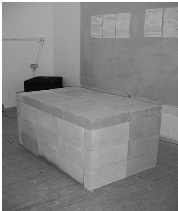
Figure 7.1 - Standard unit constructed of lightweight concrete blocks.
