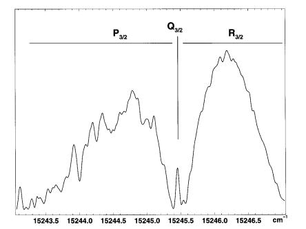
FIG. 2. Cavity ring down absorption spectrum of the  $A^2\Pi_{3/2} \leftarrow X^2\Pi_{3/2}$  electronic origin band of NC<sub>6</sub>N<sup>+</sup>, recorded through a supersonic plasma. The second spinorbit component is not visible at the low temperature in the jet ( $T_{\rm rot} \sim 15$  K). The *Q*-branch position is used to assign the FPM spectrum.
