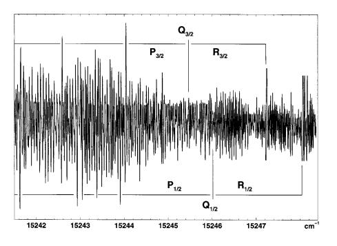
FIG. 1. Rotationally resolved frequency production double modulation absorption spectrum of the  $A^2\Pi_u \leftarrow X^2\Pi_g$  electronic origin band of NC<sub>6</sub>N<sup>+</sup> measured in a liquid-nitrogen cooled hollow cathode discharge ( $T_{\rm rot} \sim 150$  K). The *P*-, *Q*- and *R*-branches of the  $A^2\Pi_{3/2} \leftarrow X^2\Pi_{3/2}$  and  $A^2\Pi_{1/2} \leftarrow X^2\Pi_{1/2}$  subbands are indicated.
