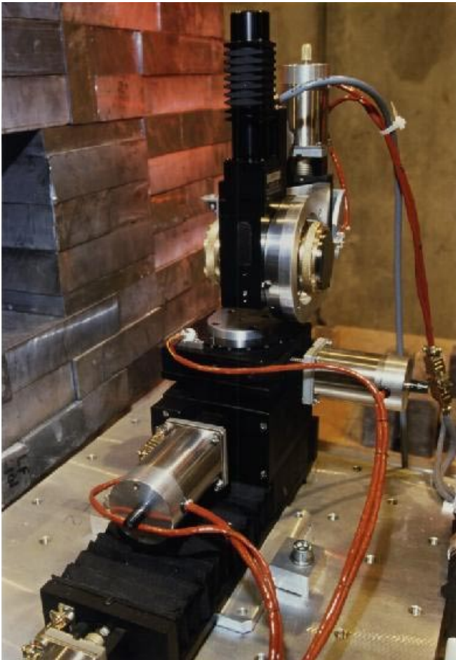
FIG. 10. (Color) Birefringent (quarter wave plate) Si crystal and goniometer.
