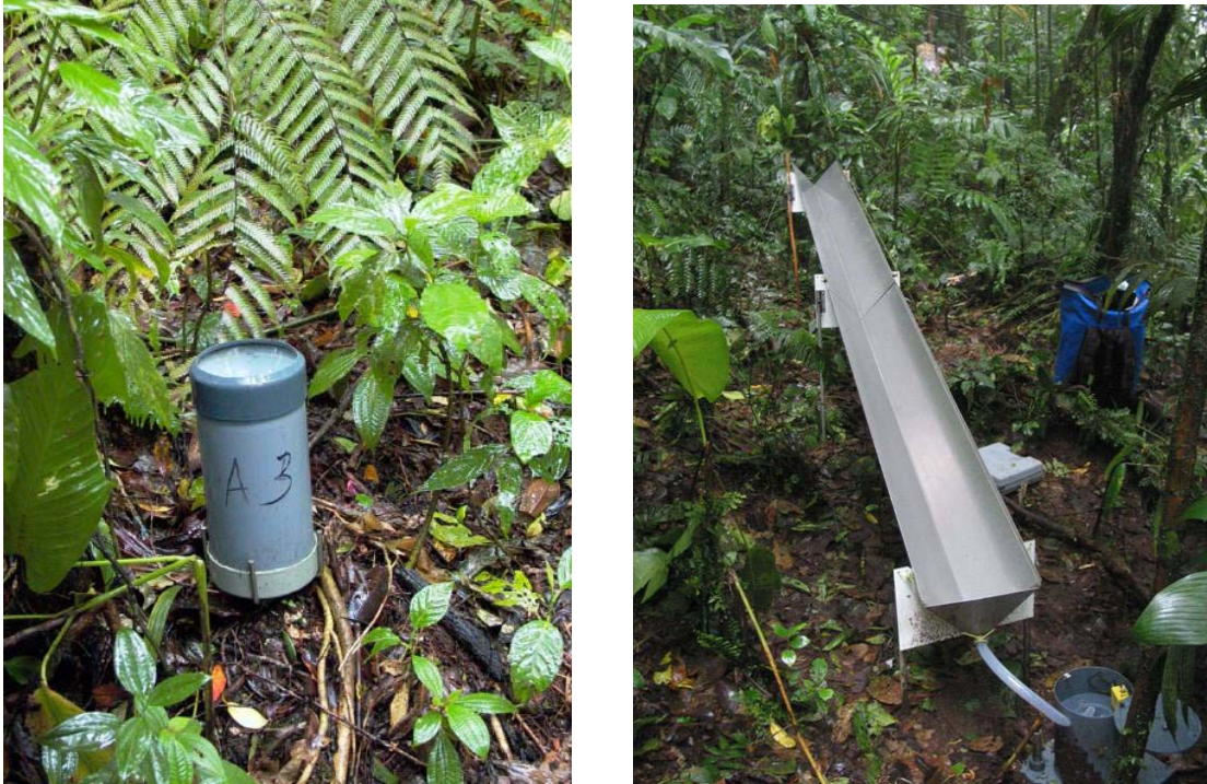
Figure II.14, (a) Manual throughfall gauge placed in metal holder. (b) Throughfall gutter connected to tipping- bucket recorder system.
