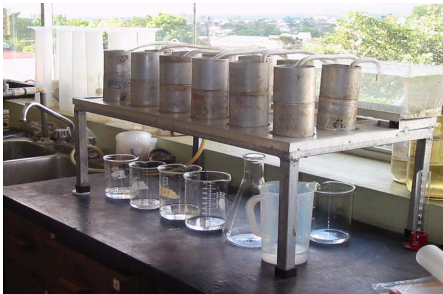
Figure IV.5. Table siphon system to determine saturated soil hydraulic conductivity through the constant-head method.
