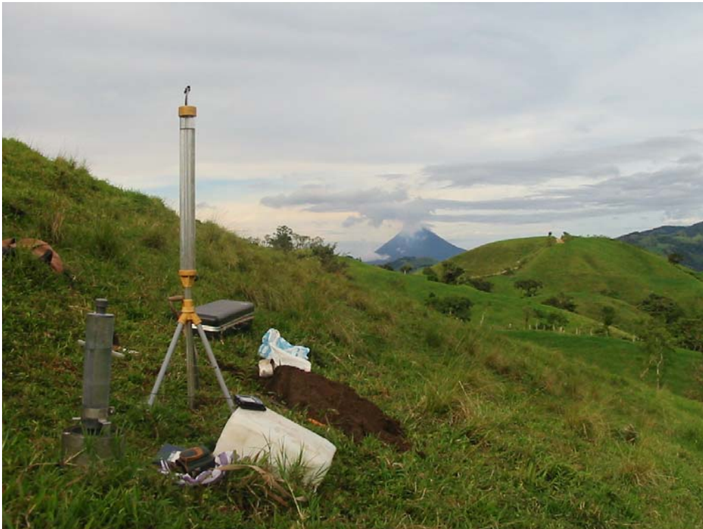
Figure IV.6. Field determination of saturated hydraulic conductivity using the Guelph Permeameter.
