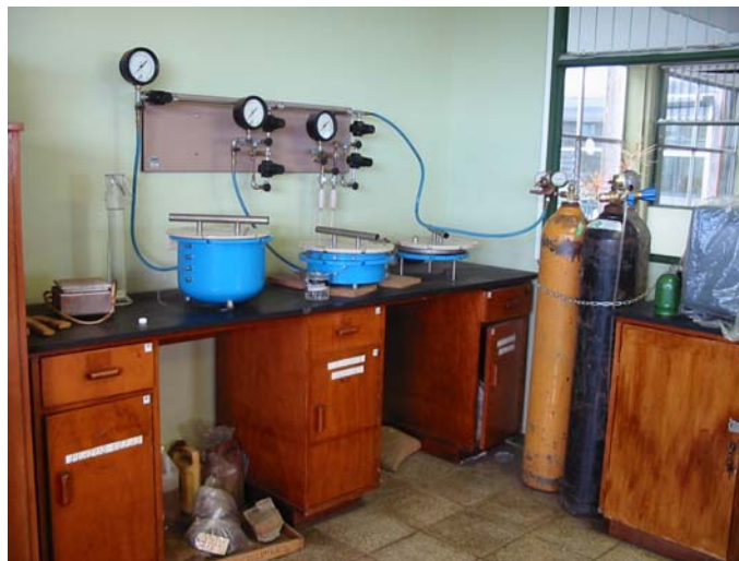
Figure IV.4. Pressure plates for determination of water retention characteristics at high tension values.
