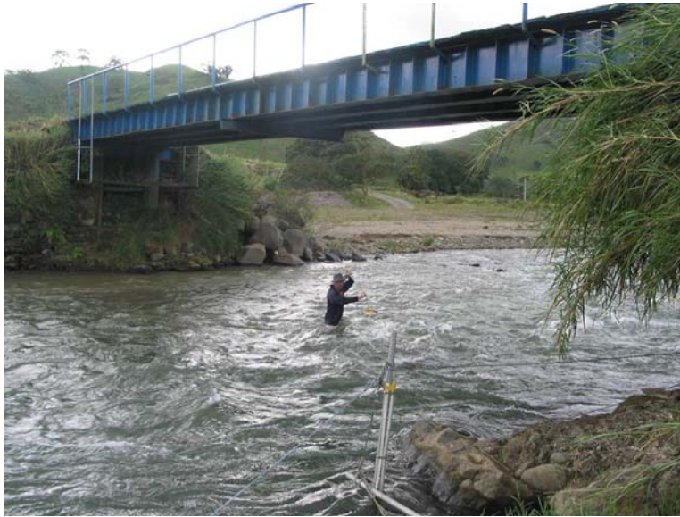
Figure V.7. Manual streamflow velocity measurement using a current-meter.
