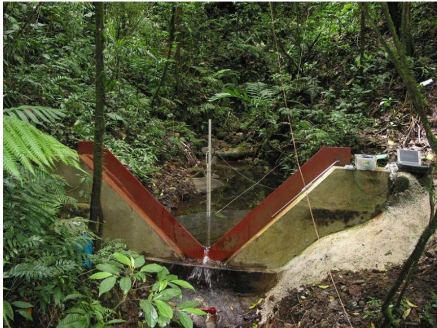
Figure V.4. Sharp-crested V-notch weir as used to gauge the project's micro-catchments.
