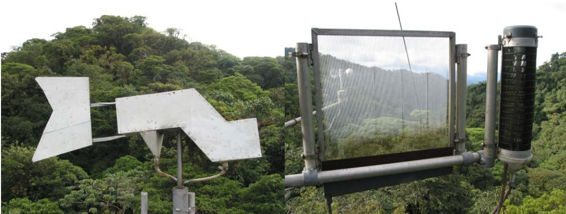
Figure II.7. Passive fog gauges, from left to right: rotating Daube tunnel gauge, wire harp, and modified Juvik-type fog gauge as installed on top of a scaffolding tower to allow measurements to be made above the cloud forest canopy.
