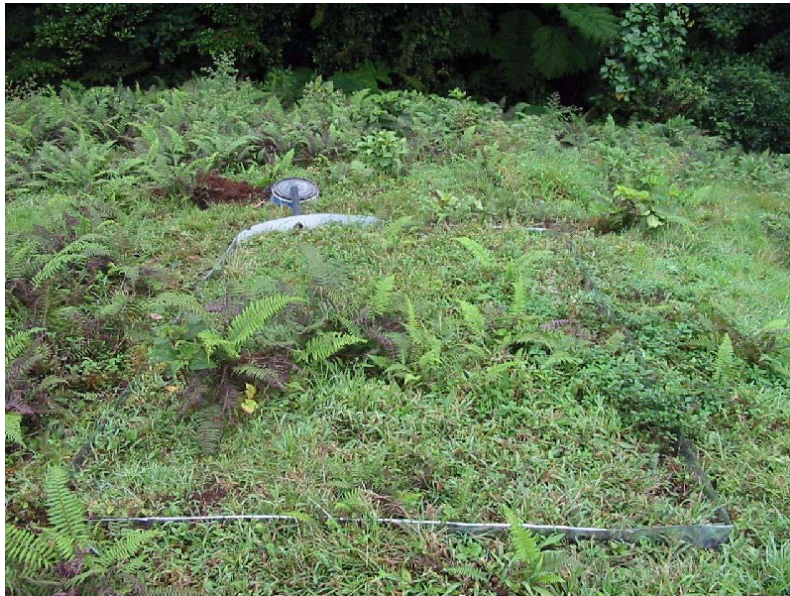
Figure IV.14. Bounded plot for surface runoff measurements in a pasture formerly occupied by cloud forest. Note runoff collection tank at downslope end and sheet metal boundaries.
