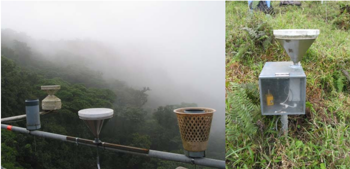
Figure II.2. Left-hand panel: Different types of rain gauges installed on top of a 25 m high scaffolding tower extending above the cloud forest (canopy height 20-22 m). From left to right: standard manual gauge, Campbell ARG100 automatic rainfall recorder, custom-built VUA rainfall recorder, and shielded standard rain gauge. Right-hand panel: Custom built VUA recording gauge with tipping bucket and data-logger installed inside a pvc-box with funnel fitted on top.
