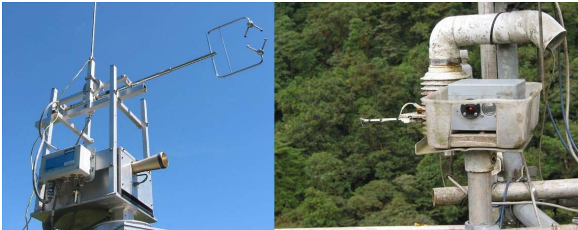
Figure II.11. (a) Eddy-covariance set-up consisting of FM-100 cloud droplet spectrometer and Gill Solent sonic anemometer (top right). (b) Optical fog sensor (OFS-Mk2) placed inside a simple plastic box (cover temporarily removed) to protect laser window (red) and adjacent detector window from direct deposition of wind-driven droplets.
