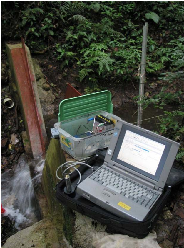
Figure V.13. Diver DI240 water level sensor (temporarily taken out of installation tube shown in background) and laptop computer placed on top of sharp-crested weir during downloading of stage data.
