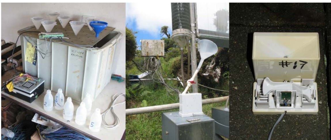
Figure II.6. Left: Calibration of tipping buckets (type WS7048) at the field laboratory Santa Elena, Costa Rica; centre: in situ calibration in the field; right: close-up of tipping bucket.
