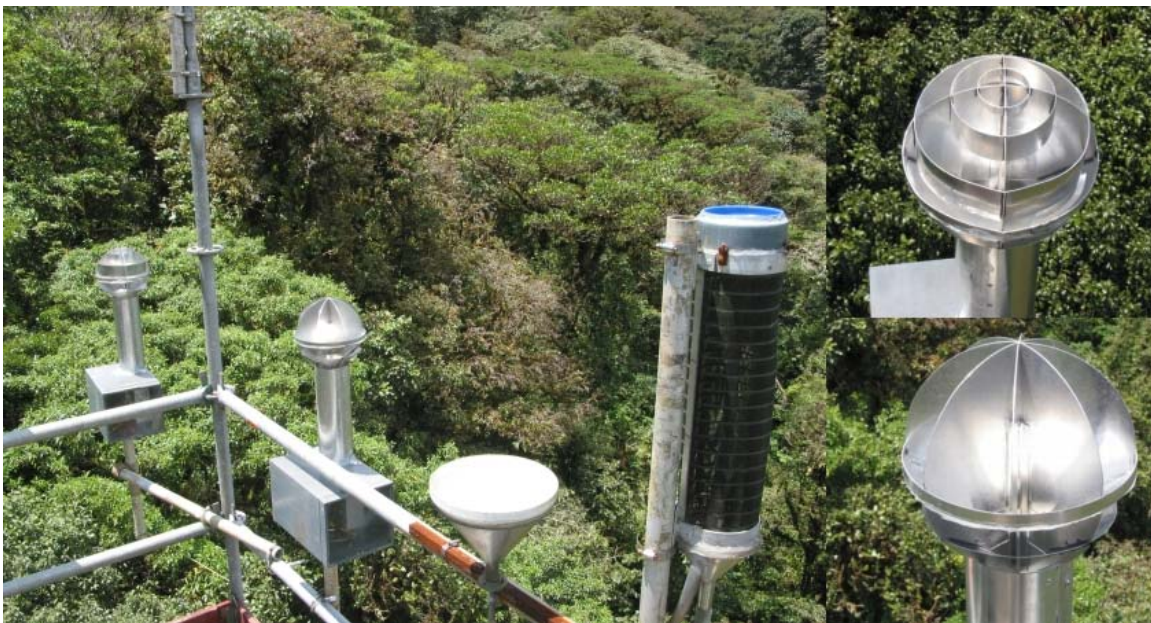
Figure II.3. Spherical rain-gauge experiment. Installation on top of the tower (left) and detailed view of spherical gauges using cylinders (right top) and vanes (right bottom). Also shown (centre) is a modified Juvik cylindrical fog gauge used for the evaluation of potential precipitation.
