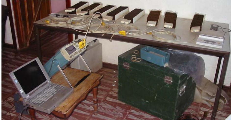
Figure 13. PVC molds for calibration of TDR sensors and set-up at field station..
