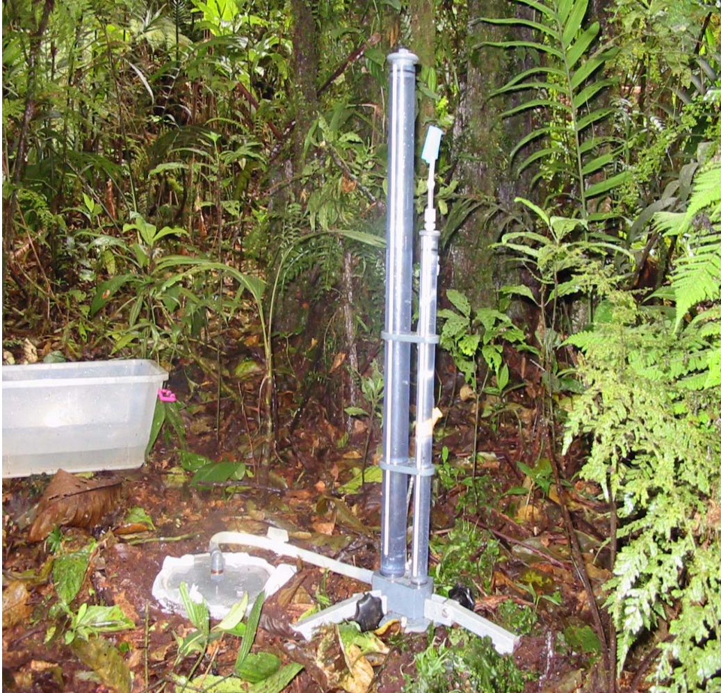
Figure IV.9. Tension-infiltrometer to derive unsaturated hydraulic conductivity k(h) in the field showing ceramic disk (left), water reservoir (centre) and bubble tower (right).
