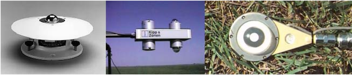
Figure III.11. Pyrgeometer (Eppley-PIR, left) and two net radiometers (CNR1, middle) and (Q7, right).
