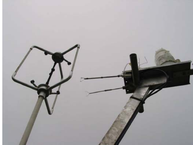
Figure III.4. Left: Sonic anemometer (Gill Solent Instruments, model R2) . Right: wet- and dry-bulb thermo-couples plus feeding reservoir .
