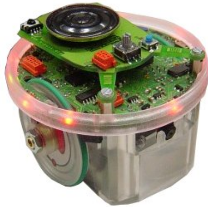
Figure 1: The e-puck robot developed at the École Polytechnique Fédérale de Lausanne (EPFL).
