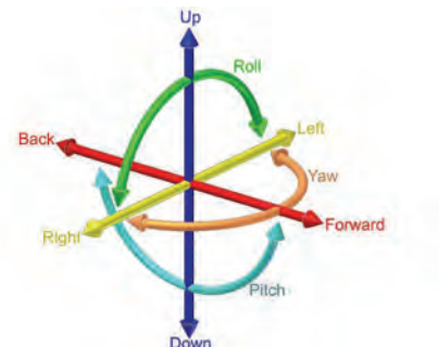
Figure1. Graphical description of movements addressed in 6DoF input devices
