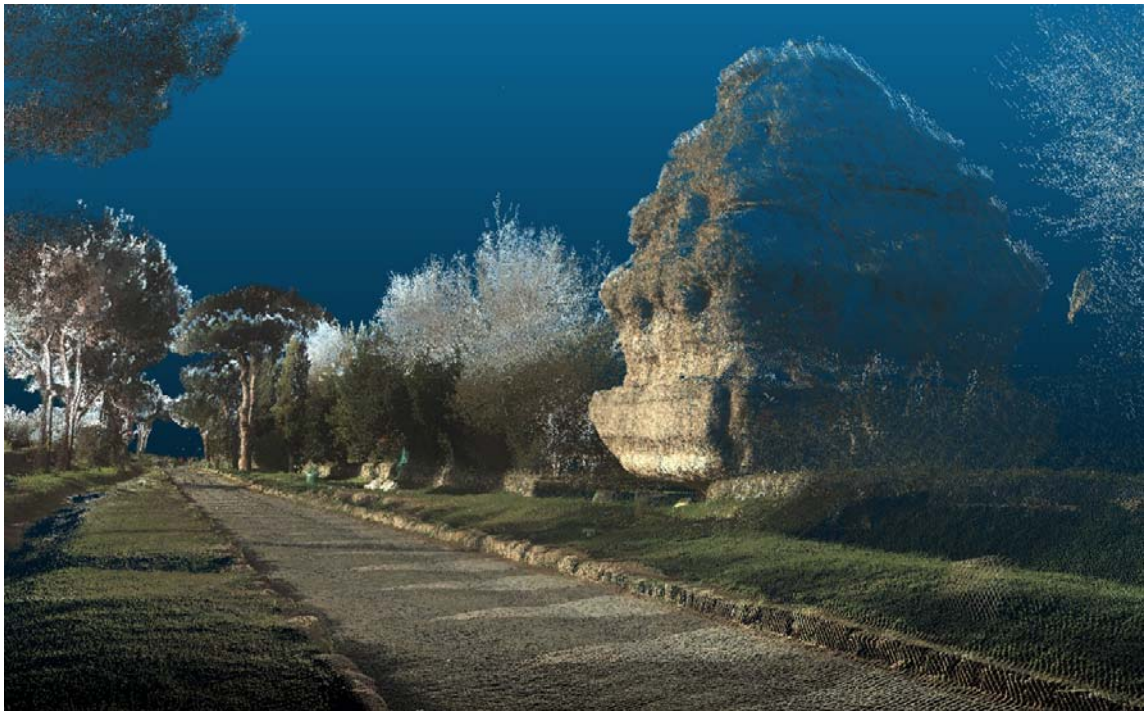
Figure 2. Point cloud measurement by Fugro's FRIVE-MAP application (figure authors).
