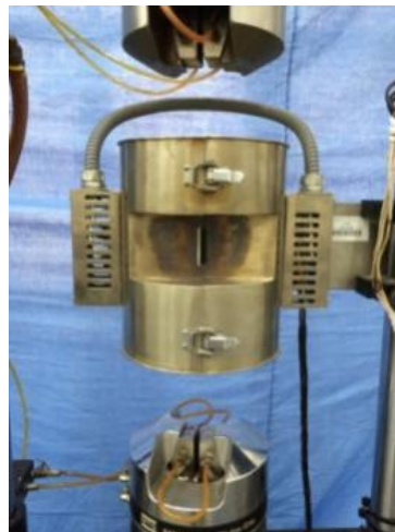
Fig. 2 High-temperature environment chamber
