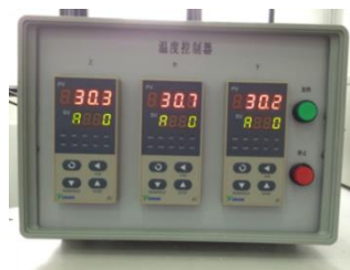
Fig. 3 Temperature controller for the environment chamber
