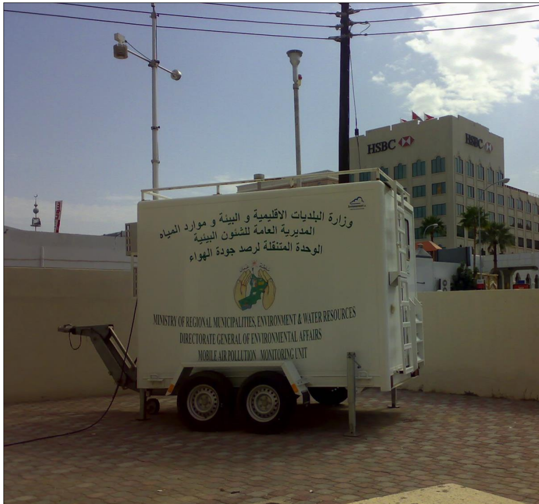
Figure II.3-3: The static air pollution-monitoring unit used by MECA. Note: although it is a mobile unit, it was kept in one place during the three years of monitoring (2007-2009).
