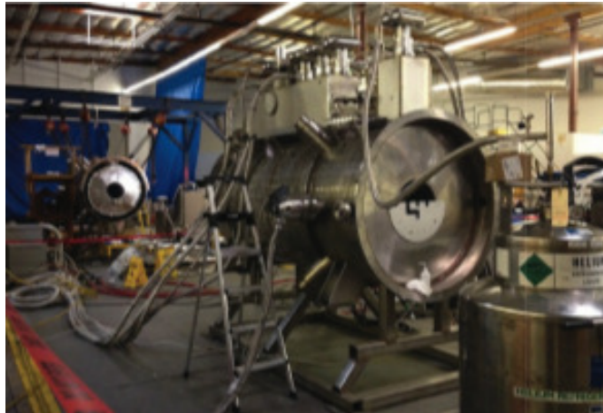
Figure 3.2: MICE spectrometer solenoids magnet. Adapted from D. Rajaram and P. Snopok, [38]
