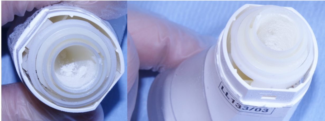
Fig. 3.16 Triboelectric effect inside the DPI hopper with blend, once the content has been poured into the Faraday Pail.
