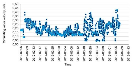
Figure 20: The circulating water velocity in the district heating connection (05.02.2012 - 07.04.2012)
