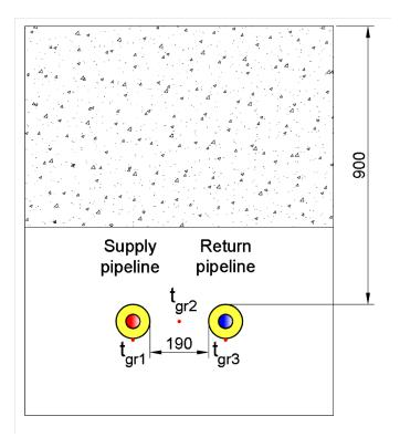
Figure 25: The locations of the ground temperature measurements (tgr1, tgr2, tgr3)
