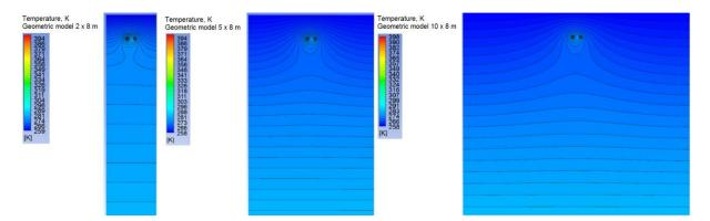
Figure 6: The ground temperature distribution for various variants of the geometric area width
