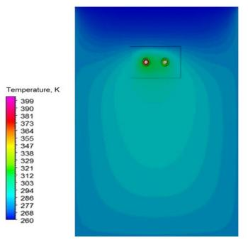
Figure 5: The ground temperature distribution in case of using the wrong types of boundary conditions
