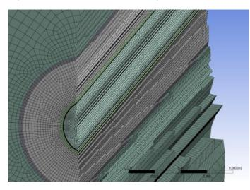
Figure 11: Hexahedral cells - the cross-section through the flow line of the pre-insulated pipe
