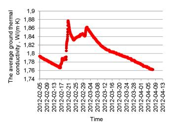
Figure 18: The ground thermal conductivity around the pre-insulated pipelines (05.02.2012 – 07.04.2012)
