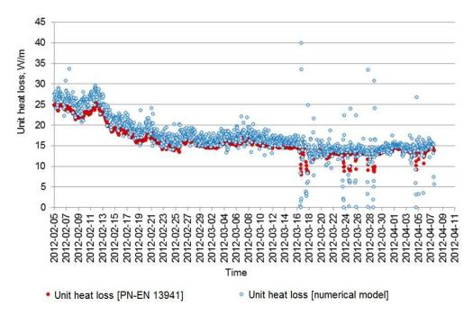
Figure 23: The outcomes of the unit heat loss calculation in the flow pipe based on the PN-EN standard guidelines and computation with the numerical model
