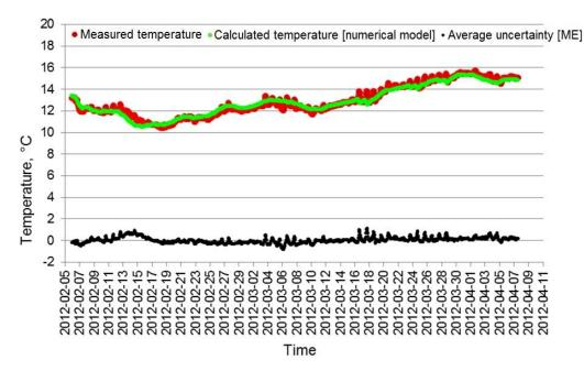
Figure 27: The outcomes of the measurements and calculation of the ground temperature in point  $(t_{gr2})$
