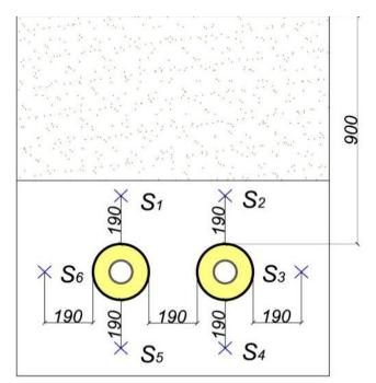
Figure 16: The ground volumetric moisture measuring probe location around the pipeline
