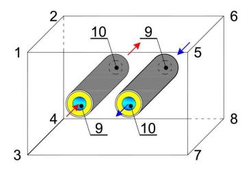
Figure 21: Scheme of the boundary conditions indication in the three dimensional computational model
