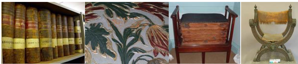
Figure 1: examples of historic leather artefacts suffering from acid-deterioration (courtesy of Karen Vidler and The Leather Conservation Centre, Northampton, UK).
