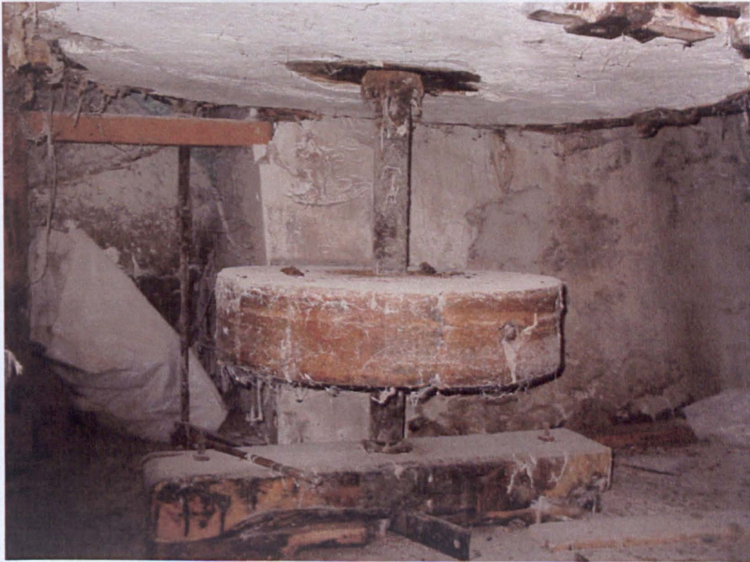
Figure 5. 89. Millstone, spindle and pivot inside mill house of BU0049. (Photo: Chris Parks)
