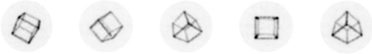
Figure 2. Projected 3D cube, created using 120 output points, generated at the distal end of the MMF with a refresh rate of 50 Hz. The contrast ratio of the cube lines to the fibre background light is 20 : 1. Colours are inverted.
