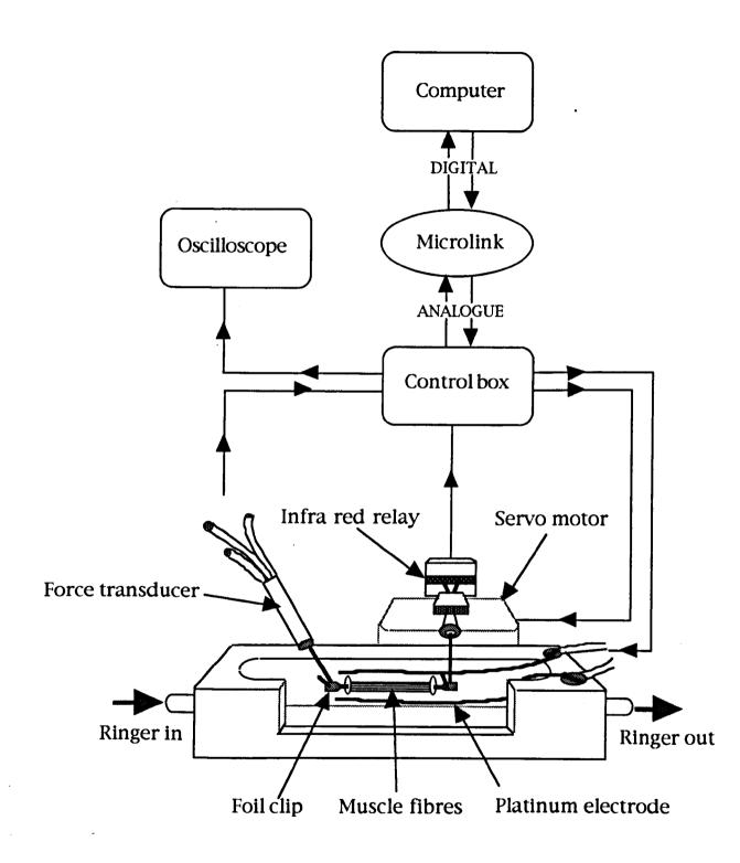
The experimental system was designed to calculate the work done by an isolated fibre bundle under varying conditions of length and activation. The system consisted of four main sections (fig. 2.2):
