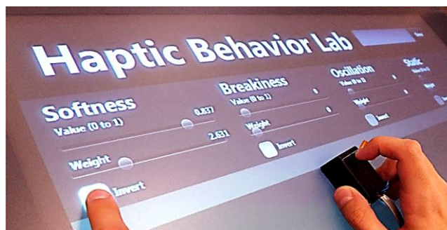
Figure 1. Behavior Lab lets developers explore, combine and feel diverse haptic behaviors before writing code.
