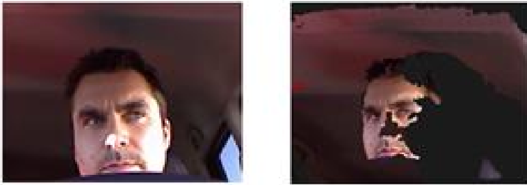
Figure 6-12: Excessive lighting reflected saturates the sensor
