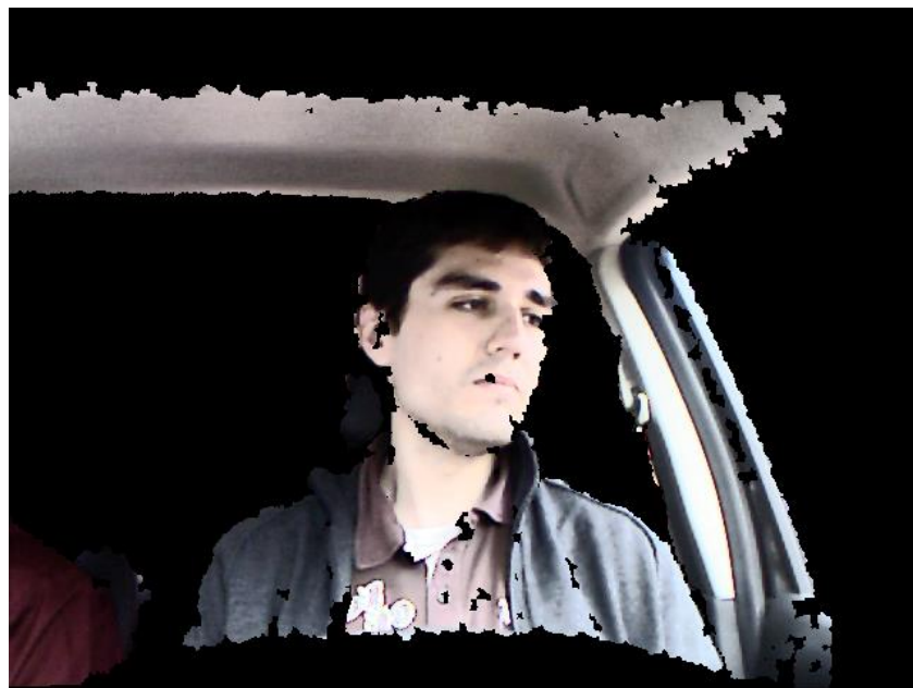
Figure 6-19: Occlusion of the left eye and high presence of invalid data
