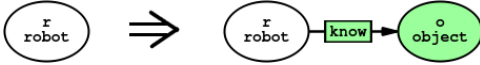
Fig. 3. Example of a graph transformation rule used to make the robot find new objects.
