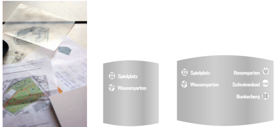
fig. 126 - fig. 128 example for direction signs made of stainless steel - draft and testing mock-up (original size model made from card- board)
