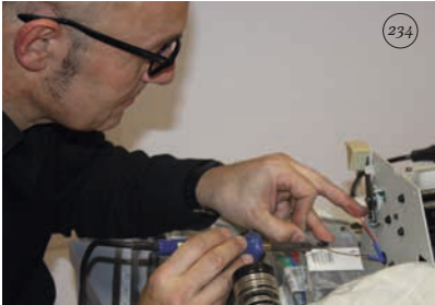
fig. 234 After only a short working time the new cutting machine had a technical defect. Once soldered the spare parts, the vinyl-cutter continued to operate for the next weeks
