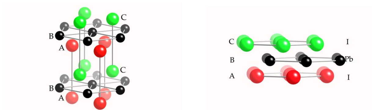
Fig. 3 The ABC structure of the 2H polytype of \text{PbI}_2 . For convenience, one layer of I atoms is red and the other layer is green, as in Fig. 2. The hexagons and triangles in the plane and the lines in the z -direction are guides for the eye. Coordinates from ICSD 068819 which are from [23]. (a) Two identical sandwiches explicitly showing the ABC structure. (b) One sandwich using just hexagons to represent the structure. This is identical to the bottom sandwich in all three parts of Fig. 4.
