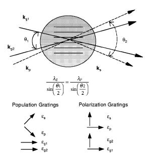
FIG. 1. TC-RFWM as a process of creating and probing laser-induced gratings.
