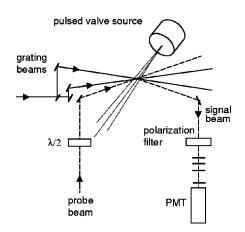
FIG. 5. Experimental arrangement used for TC-RFWM.
