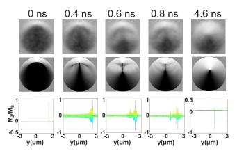
FIG. 2. (Color online) Transient domain states observed both in experiment and simulation shortly after the falling edge of a 5 mT excitation pulse (removed at time t=0 ns). The experimental PEEM images (top row) agree well with the micromagnetic simulations (second row). The cross-sectional plots of  $M_z$  along the y direction (bottom row) reveal that the vortex core is replaced by a complex cross-tie domain wall consisting of a series of cores of both positive and negative polarities.
