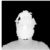
(a) Depth map example obtained from the Eurecom dataset (Min et al., 2014).
