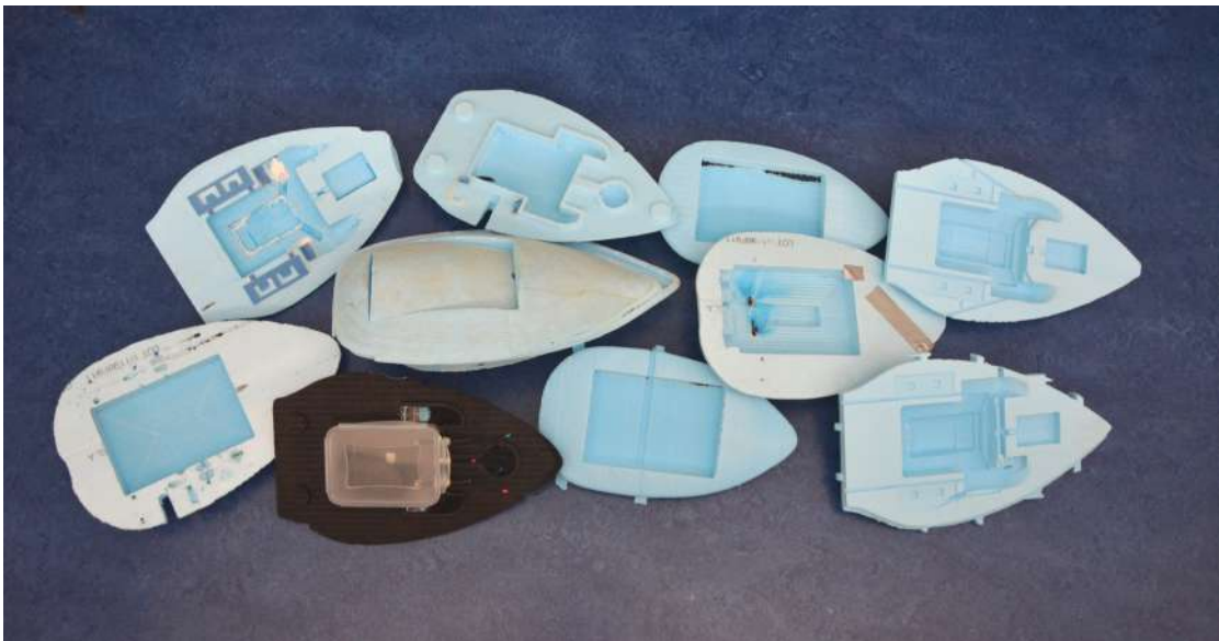
FIGURE 4.2: Different hulls produced during the design-to-product cycles. In this photography it is possible to identify the 9 different hull prototypes and the final design, on the top right.
