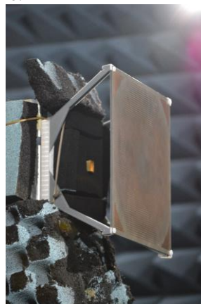
Fig. 10 – Measurement setup showing the feeding horn and the transmit-array mounted on the support.
