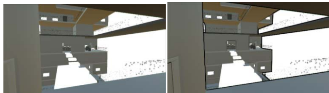
Figure 8a. No effects. Figure 8b. Sobel depth operator.
