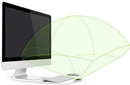
Fig. 1. Leap motion controller detection zone
