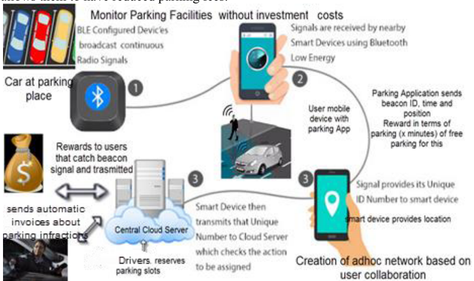
Figure 1. Overview of proposed approach to create a parking monitoring facility without investment costs using an ad hoc network of user mobile device collaborative process.
