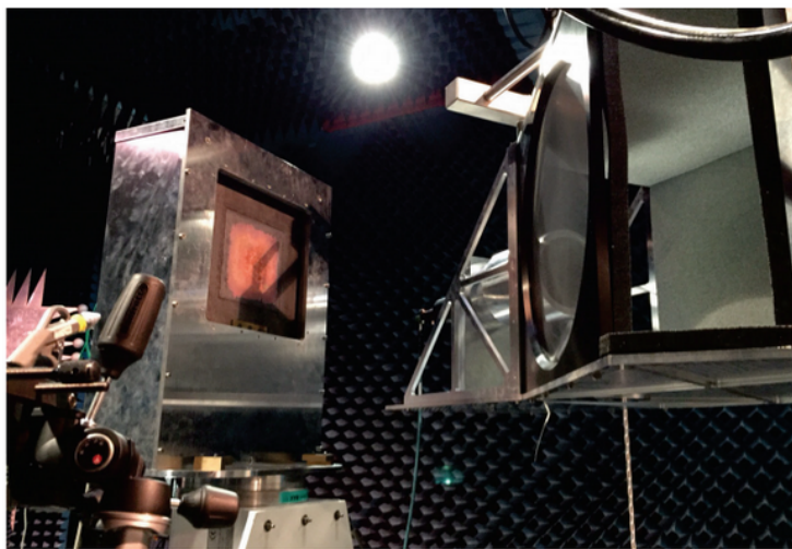
Figure 4.2: High temperature sample holder setup in Microwave test facility .
