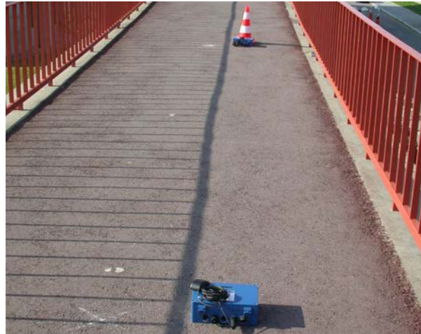
Figure 4.24 Seismograph and external GPS
