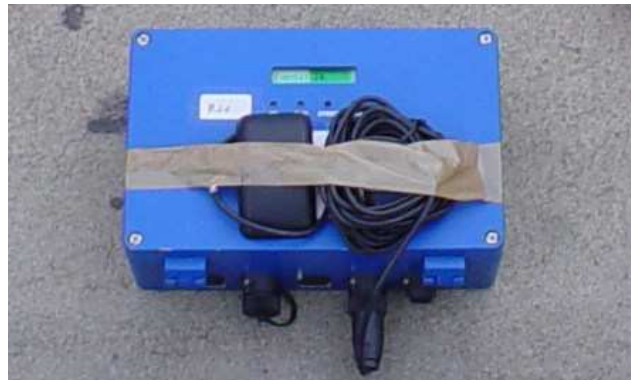
Figure 4.4 Seismograph and external GPS
