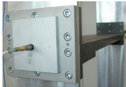
(b) Sensor (PCB 352C68) at node 2
