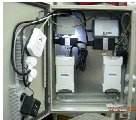
(b) NI Ethernet, DAQ devices, power-line bridge and switch
