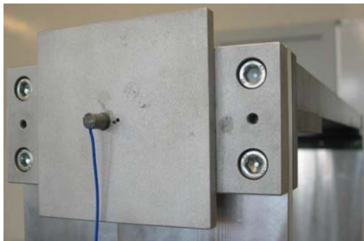
(a) Sensor (PCB 352A10) at node 1
