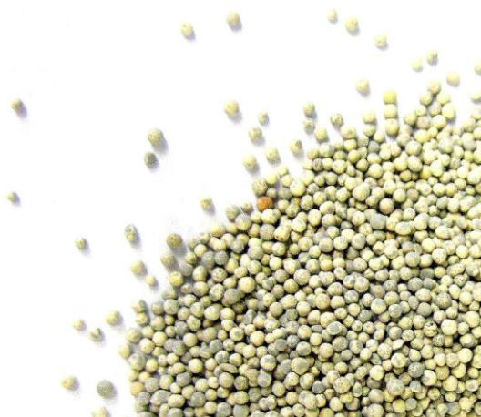
Figure 1.7 – AgLiLSX-type zeolite (sample from AirProducts).
