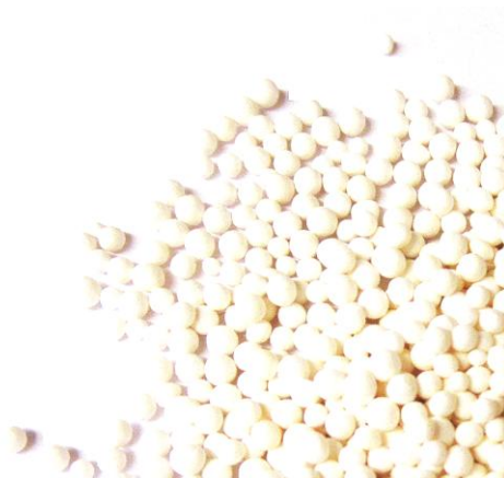
Figure 1.9 – Activated alumina (F200 7x14 Tyler Mesh, sample from BASF).
