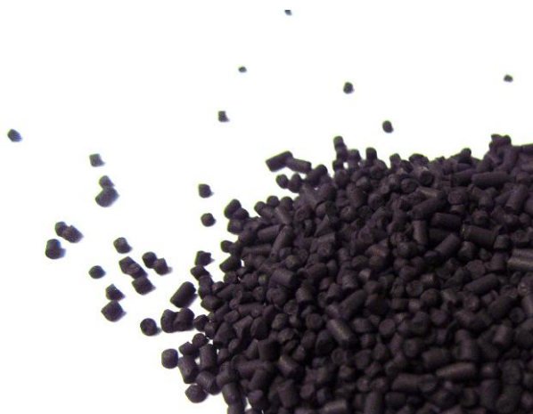
Figure 1.10 – Carbon molecular sieve (CMS-D, sample from Carbotech).
