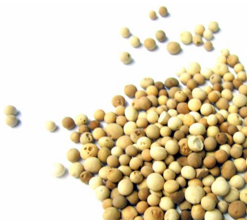
Figure 1.8 – Silica (KC-Trokenperlen WS 2050, sample from BASF).
