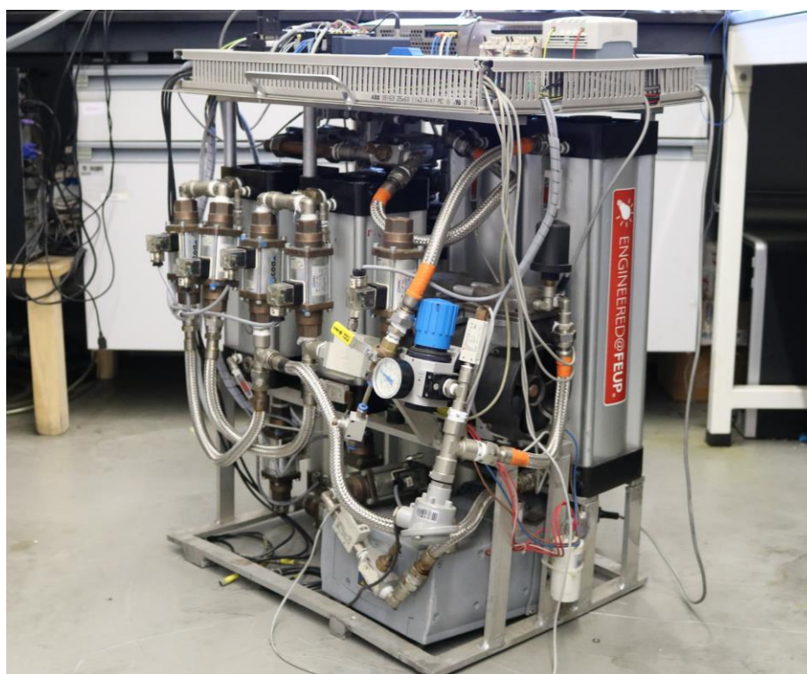
Figure A.6 – Picture of the VPSA prototype.
