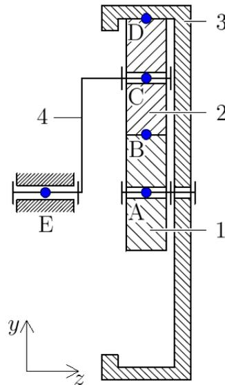
Figure 5.1.: Schematic representation of the planetary gear (side view).
