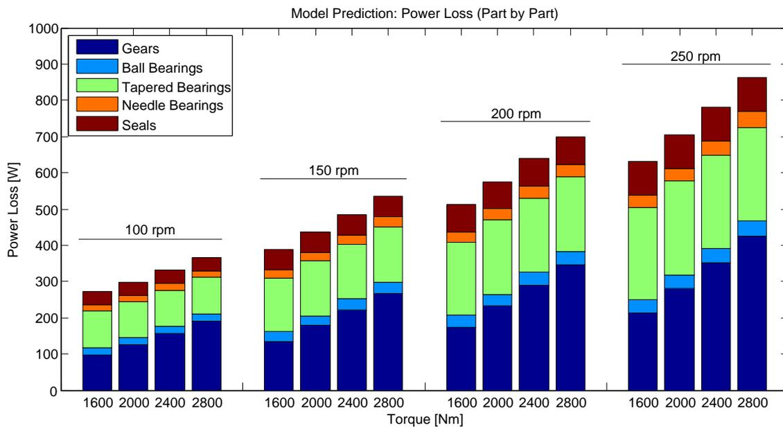
Figure 6.7.: Power Loss: Part by Part.
