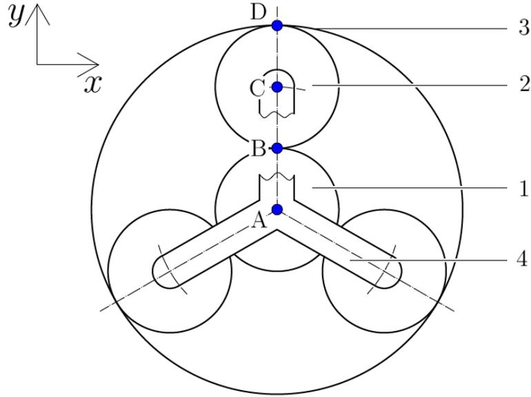
Figure 5.5.: Schematic representation of the planetary gear (front view).
