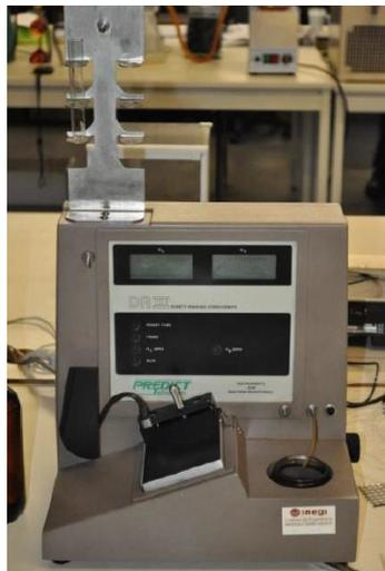
Figure 4.1.: Direct reading ferrograph by *Predict Technologies*.
