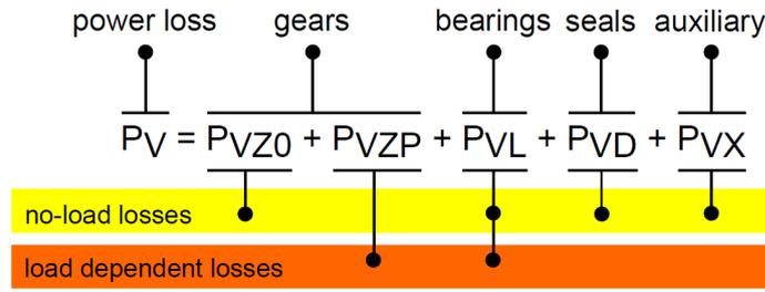
Figure 5.6.: Different power loss components in a gearbox [10].
