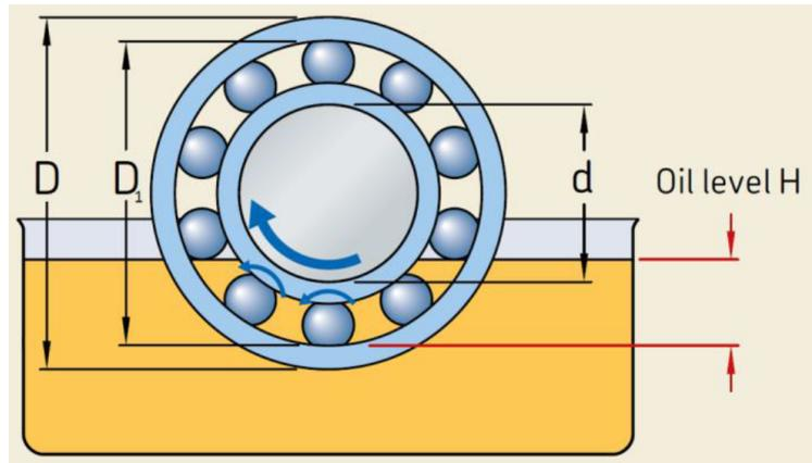
Figure 5.10.: Oil level measurement [36].
