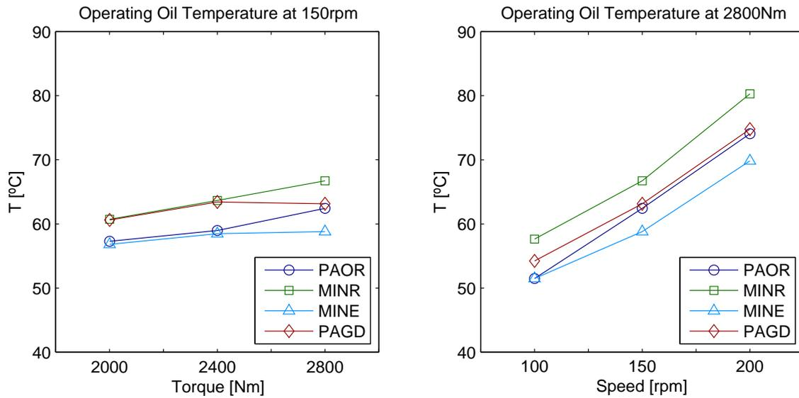
Figure 7.14.: Oil comparison: Operating Temperature.
