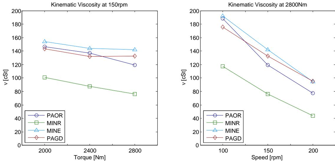
Figure 7.15.: Oil comparison: Kinematic Viscosity.
