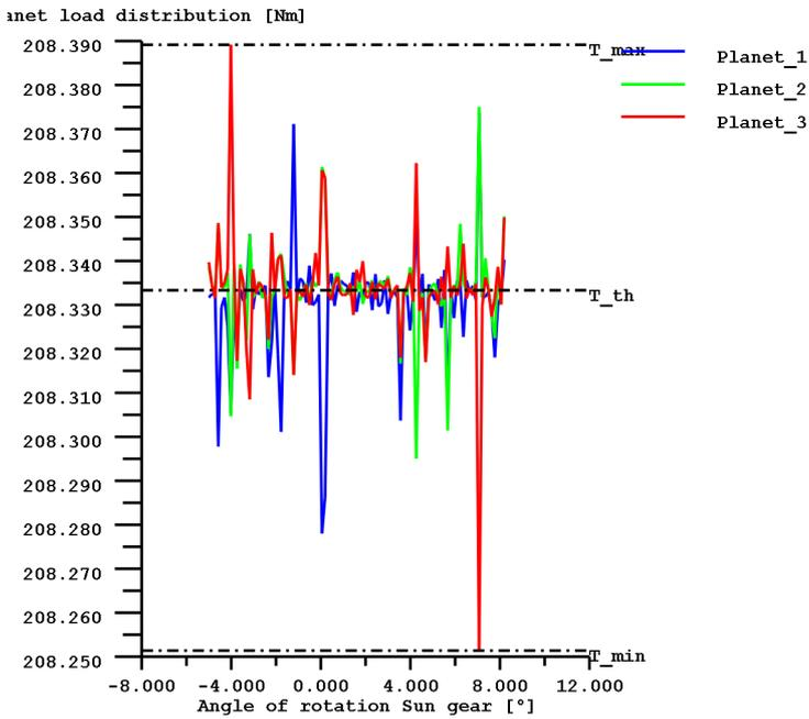
wt = 100 %, a = 73.035 mm, fpt1 = 0.000  $\mu\text{m}$ , fpt2 = 0.000  $\mu\text{m}$ ,  $\mu_1 = 0.05$ ,  $\mu_2 = 0.05$
