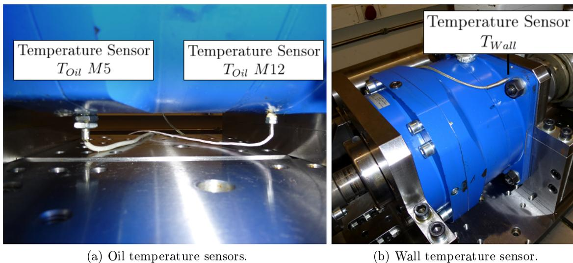
Figure 3.4.: Temperature sensors' positioning in the tested gearbox.
