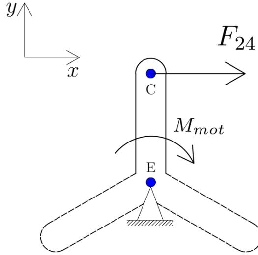
Figure 5.2.: Free body diagram of the planet carrier.
