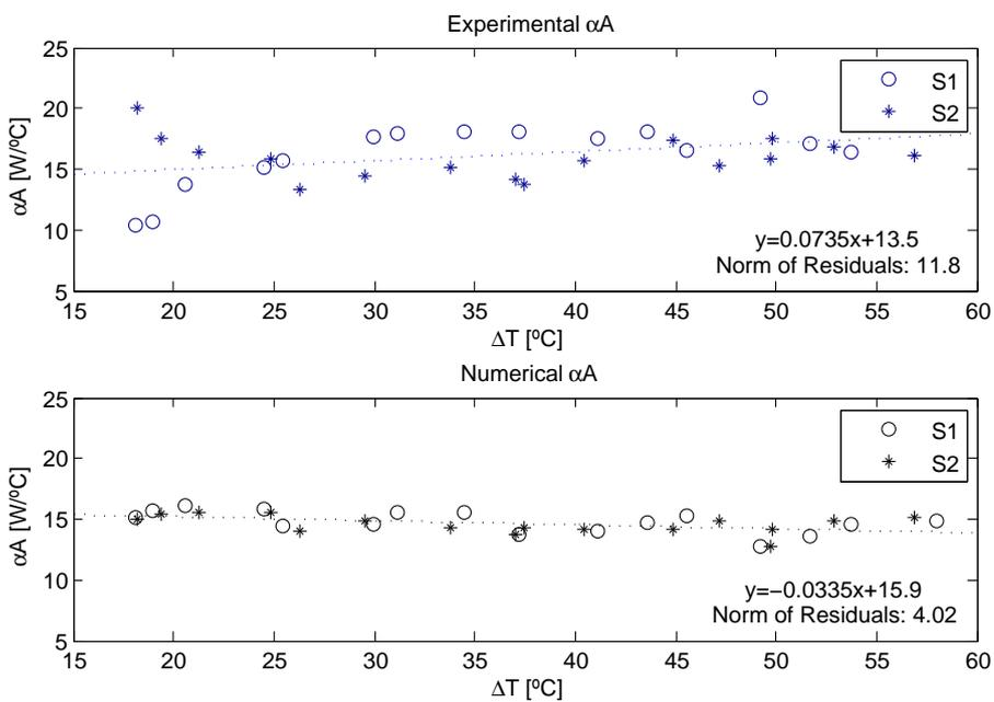
Figure 6.5.: PAOR: Heat transfer coefficient.
