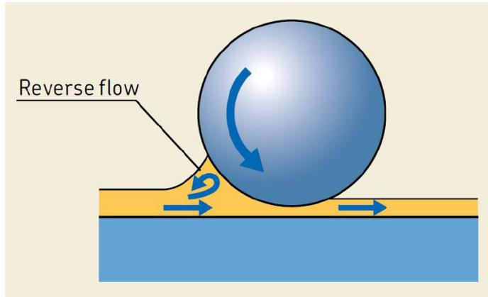
Figure 5.9.: Reverse flow in a ball bearing [36].
