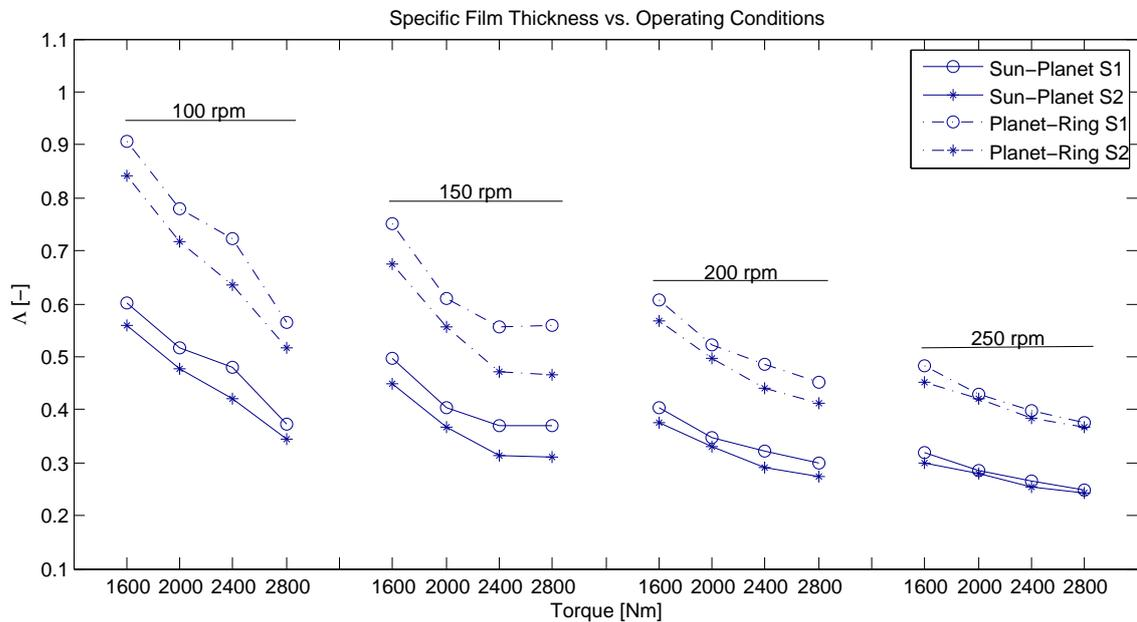
Figure 6.6.: PAOR: Specific Film Thickness.
