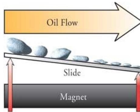
Figure 4.2.: Sedimentation process of the particles in the ferrogram [22].
