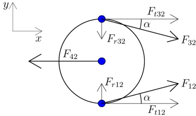
Figure 5.3.: Free body diagram of the planet.
