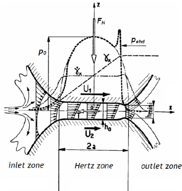
Figure 5.8.: Linear elastohydrodynamic contact [25].
