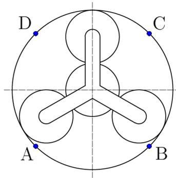
Figure A.1.: Thermocouples' positioning.
