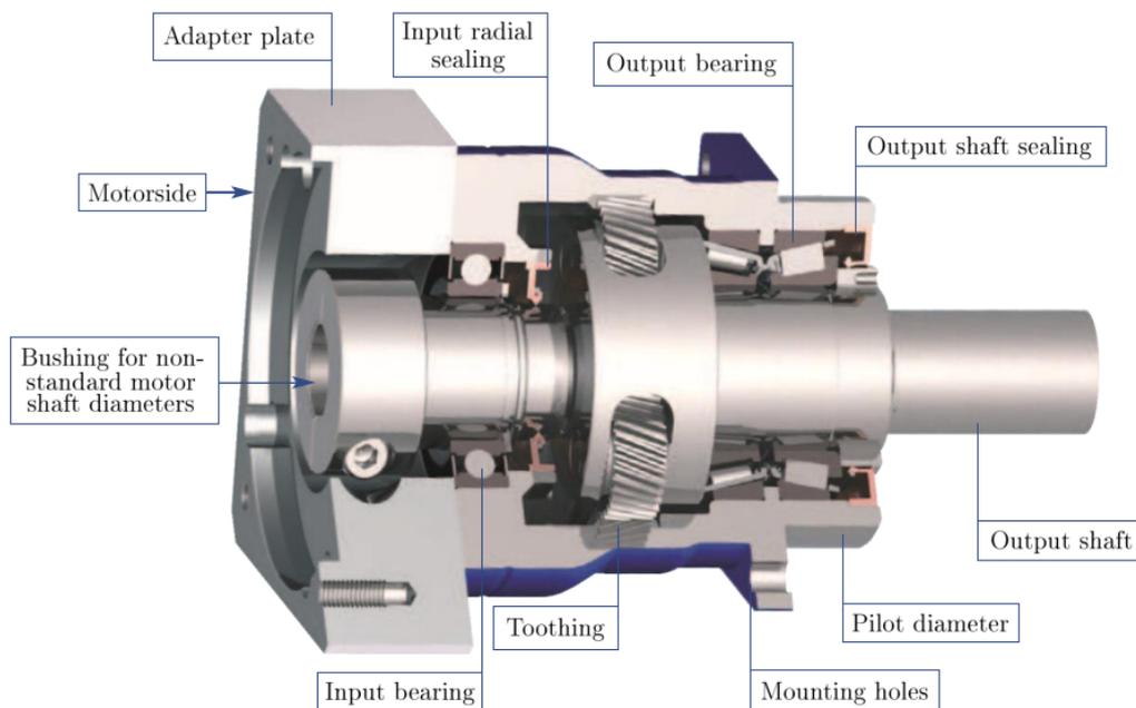
Figure 3.6.: Scheme of the planetary gearbox.
