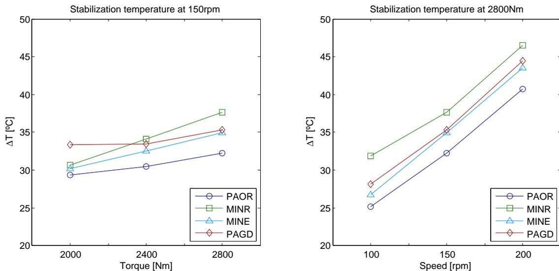
Figure 7.13.: Oil comparison: Stabilization Temperature.
