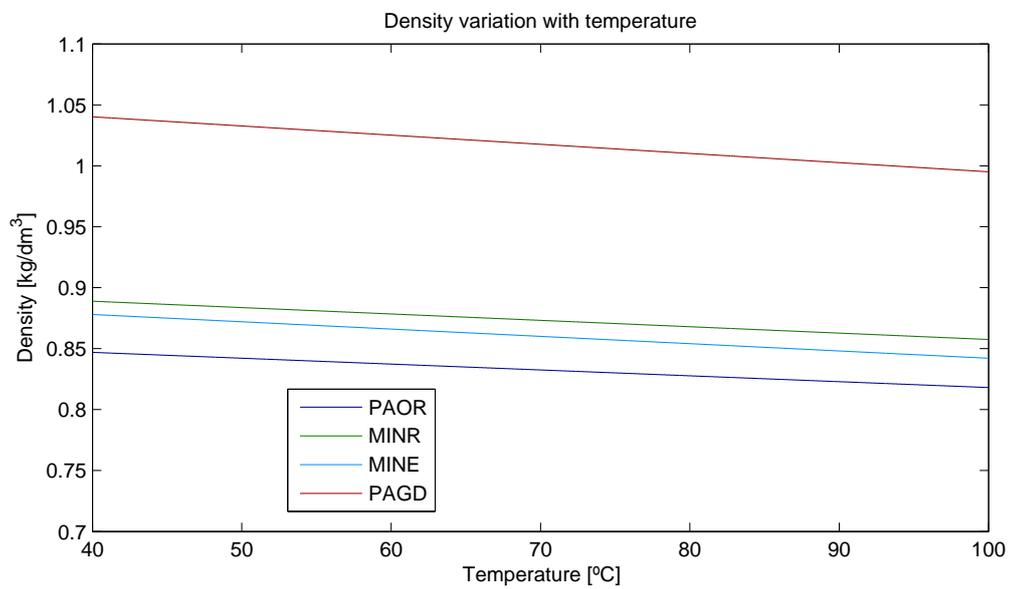
Figure 2.3.: Tested oils' density variation with temperature.
