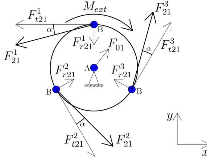
Figure 5.4.: Free body diagram of the sun.
