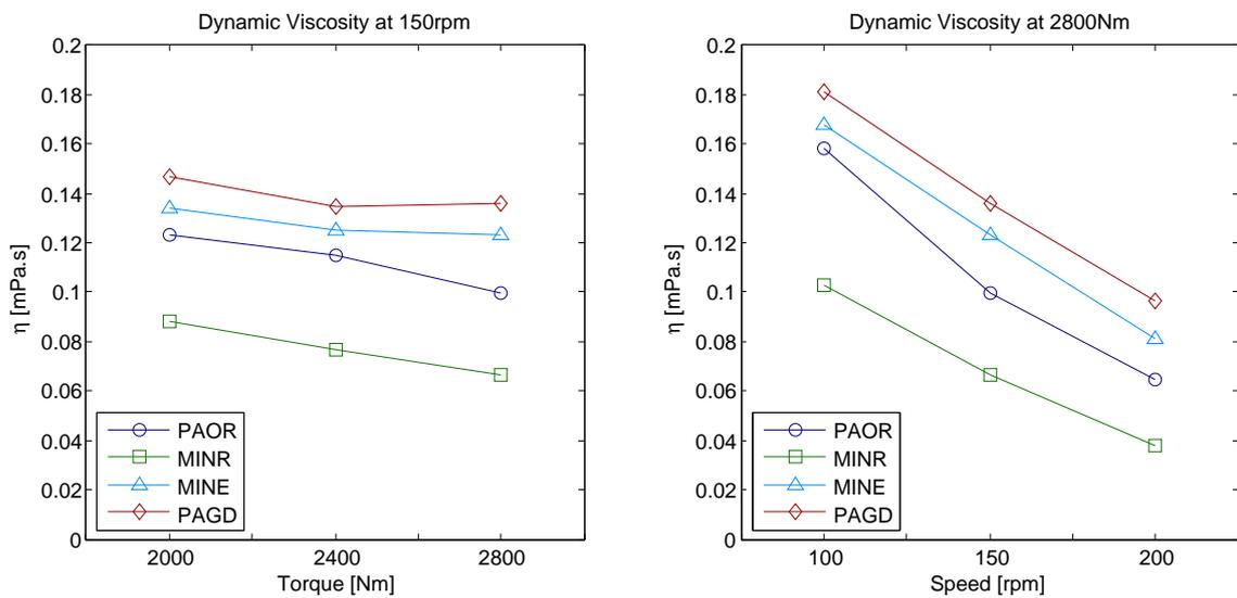
Figure 7.16.: Oil comparison: Dynamic Viscosity.
