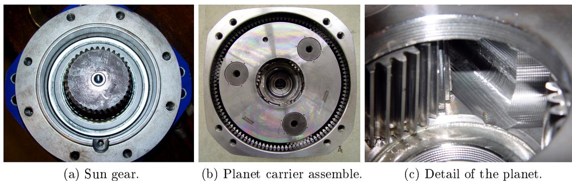
Figure 3.5.: Photographs of the tested gearbox.
