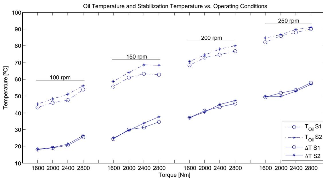
Figure 6.4.: PAOR: Oil temperature and Stabilization temperature.
