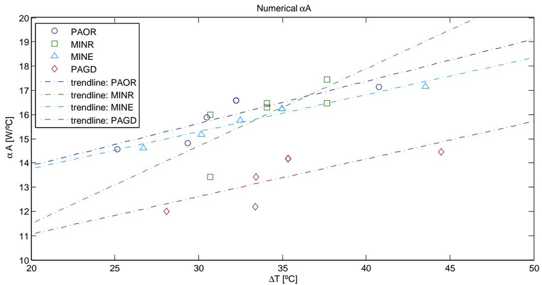
Figure 7.24.: Heat transfer coefficient: numerical values.
