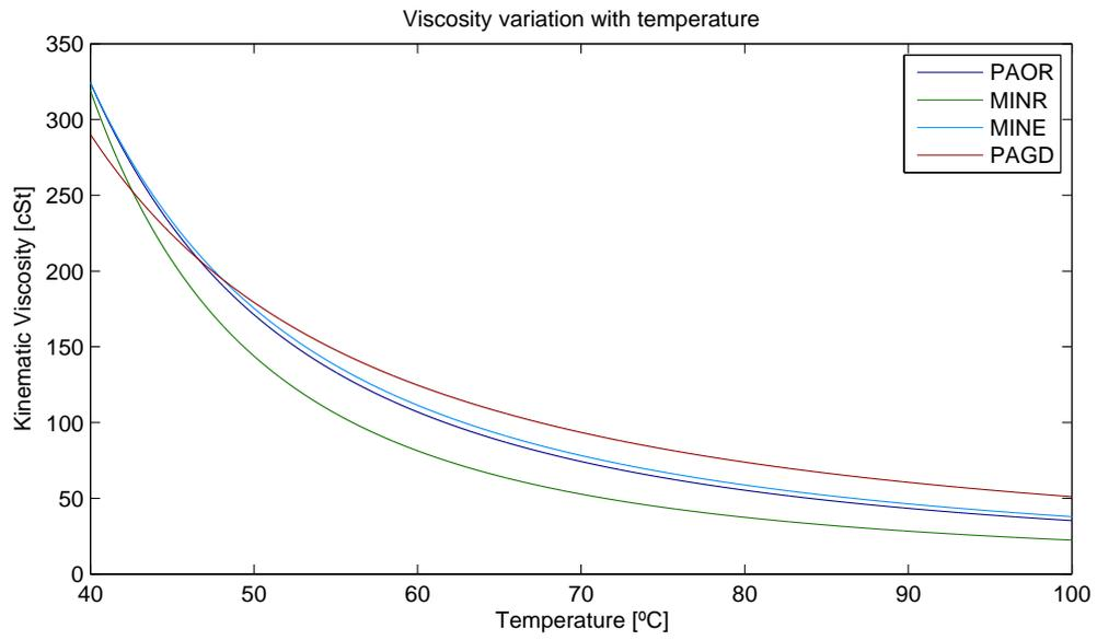
Figure 2.2.: Tested oils' viscosity variation with temperature (ASTM D341).
