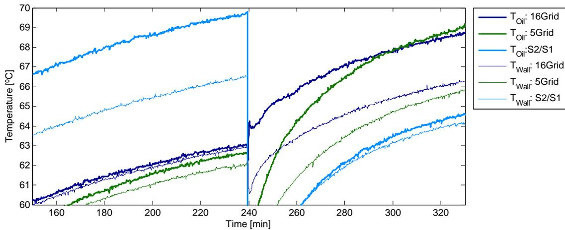
Figure 8.3.: Wall and Oil temperature evolution.
