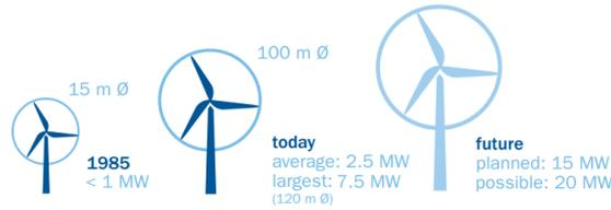
Figure 1.2.: Size and capacity of wind turbines: evolution and prediction [6].
