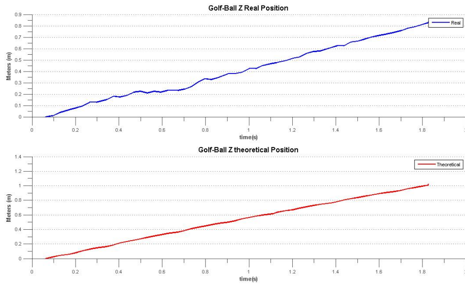
Figure 6.14: Tracings of the 3D golf-ball movement in terms of the real depth value (provided by the Kinect) and the calculated theoretical one for the slowest movement.
