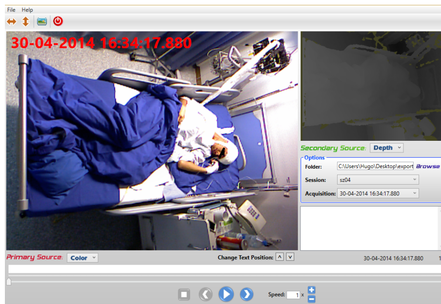
Figure 6.2: KiMA v1: Field-of-view of the Epilepsy Room. Typical distances range between 1.9m-2.1m from the sensor to the patient.
