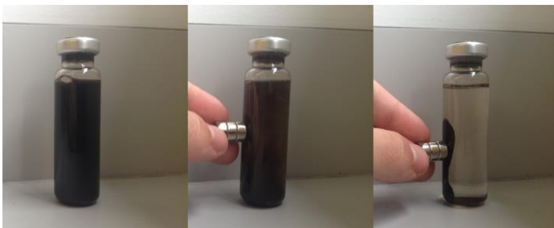
Figure 10. SPION solution response to a small permanent magnet. From left to right: the baseline suspension state prior to magnetic exposure; 1 second after the magnet's placement; and 5 seconds of magnetic influence.
