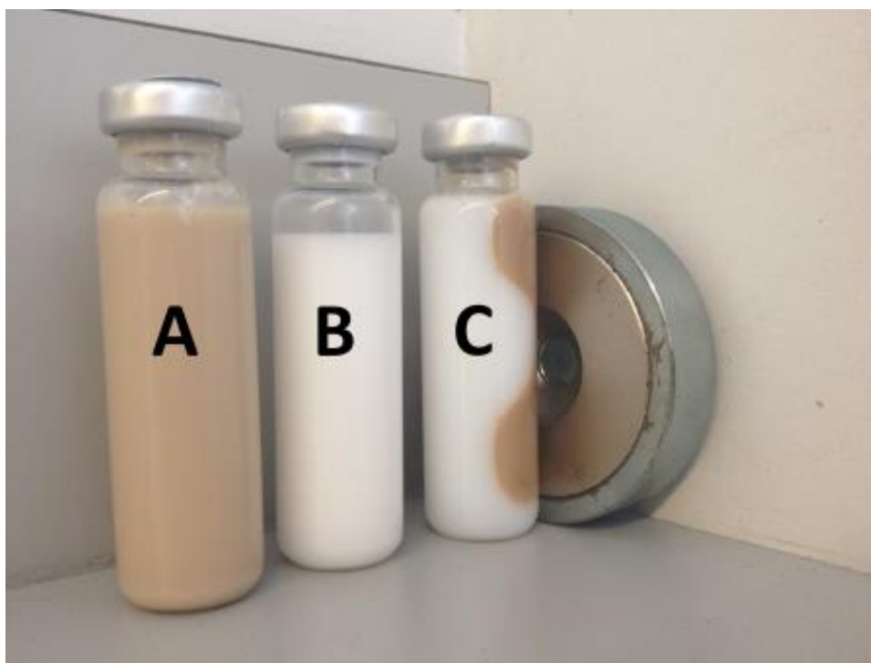
Figure 19. Comparison between the NLC-Paclitaxel-loaded (A) and Paclitaxel-loaded formulations (B) and the magnetic field influence on the first (C).
