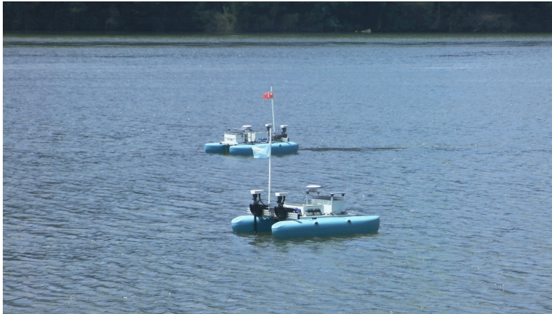
Figure 2.9: Autonomous Surface Vehicles cooperating to localize acoustic pinger in Ferreira et al. (2012).
