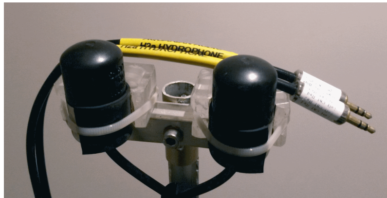
Figure 4.3: The structure holding the two hydrophones 6 cm apart.
