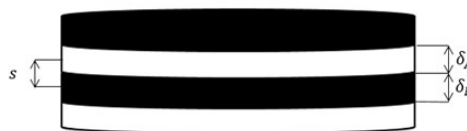
Figure 4 Striation thickness in ideal lamellar structure
