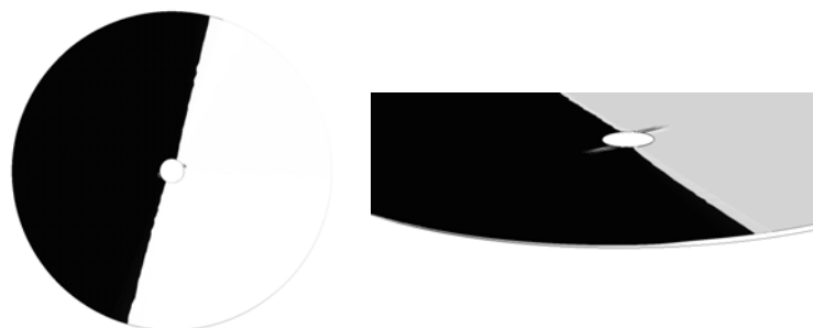
Figure 46 Result of the distribution of each fluid after one quarter of the rotation for viscosity ratio 10
