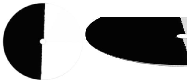
Figure 41 Cone/plate rheometer in different states of rotation for a time step of 10^{-3} one quarter of rotation
