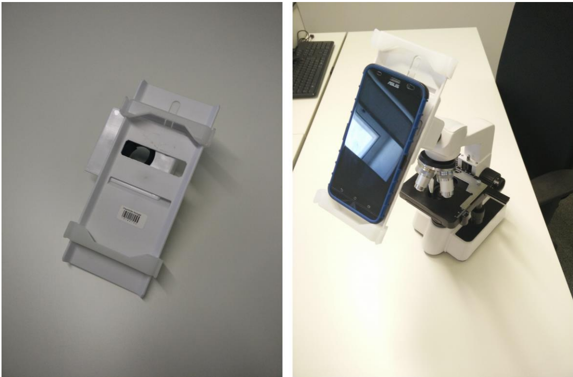
16 18 20 22 24 Figure 3.1 Skylight adaptor on the left. Skylight on microscope with mobile device ready to take pictures.
