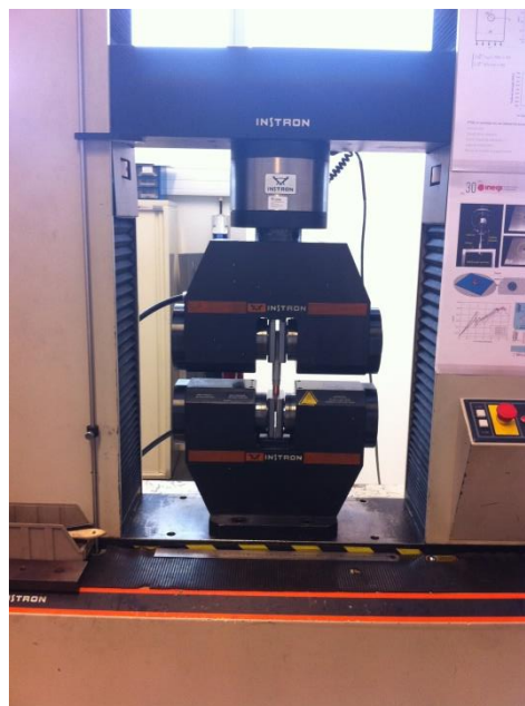
Figure 48: Setup used for the tensile tests.
