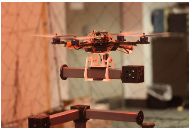
(a) Hummingbird quadcopter. source:(Lindsey et al., 2011)
