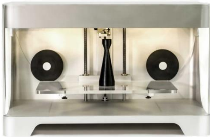
Figure 24 - Mark One Printer: The world's first 3D printer designed to print continuous carbon fiber [137]
