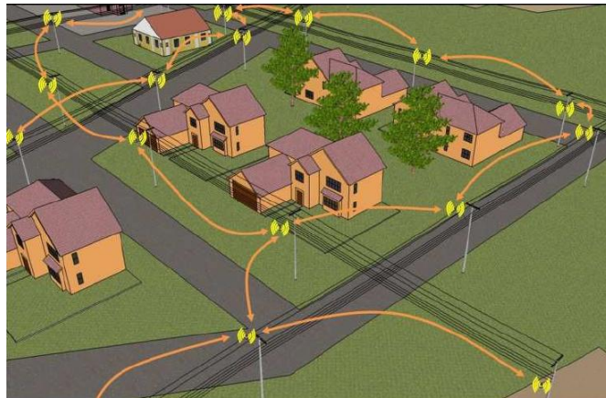
Fig. 8: Example for a meshed network [35]
