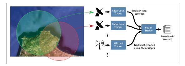
Figure 4.1: Selected processing scheme for the solution. Each sensor is processed individually, and local results are fused together by a global tracker.
