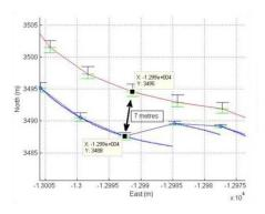
(c) Detail of UKF filter solution without 15 seconds of DGPS solution
