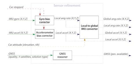
Figure 5.7: Sensor refinement module.
