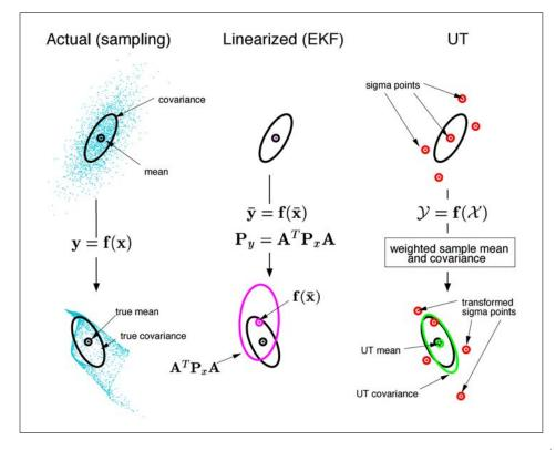
Figure A.2: Advantages of the Unscented Transform over other linearization methods. Taken from (Wan and Van Der Merwe, 2000).
