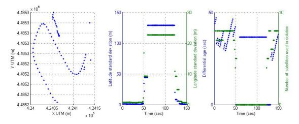
Figure 5.20: Non-underground parking area with zero satellite visibility and inactive DGPS mode using a constant value.
