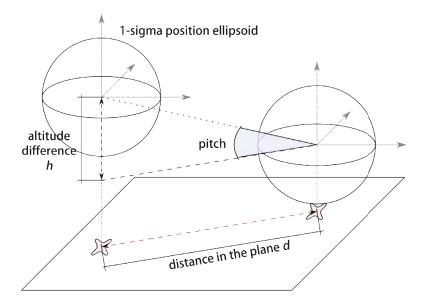
Figure 5.5: Calculation of elevation angle from two GPS measures.
