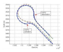
(b) DGPS trajectory (red) with deactivation and activation and UKF filter solution (blue)
