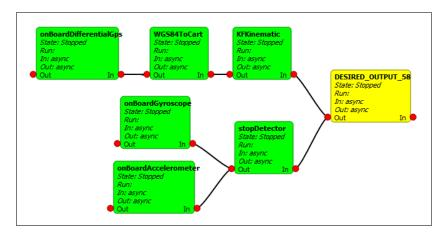
Figure 5.38: Sample fusion solution for getting high-accuracy location and stop detection
