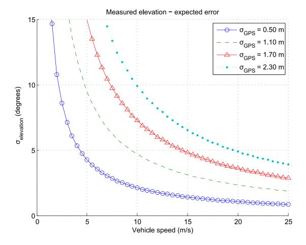
Figure 5.19: Expected standard deviation of GPS-obtained elevation angle, depending on vehicle speed and fix horizontal accuracy (simulation, 10 million iterations per point).
