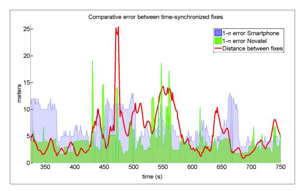
Figure 5.31: Distance between GPS fixes from Smartphone/Novatel devices, compared with the self-reported accuracy (one standard deviation).
