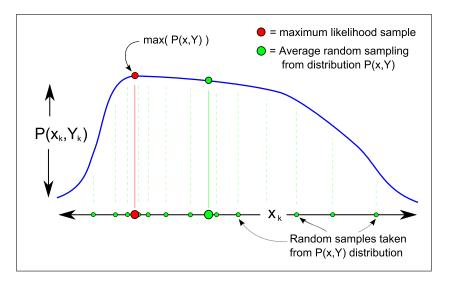
Figure A.3: State estimation calculated as the mean value of random samples, drawn according to the posterior probability distribution. Other solution, as the sample with a higher density (trying to find the peak of the real density function) offers poor results with asymmetric probability distribution.
