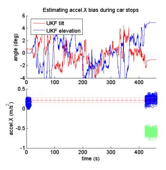
Figure 5.18: Accelerometer bias can be corrected during stops if elevation angle has been already determined.
