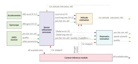
Figure 5.3: System architecture for the initial non-adaptive solution.
