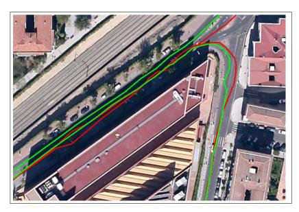
Figure 5.30: Comparison of Novatel GPS (green) and smartphone (red) raw fixes. Detail.
