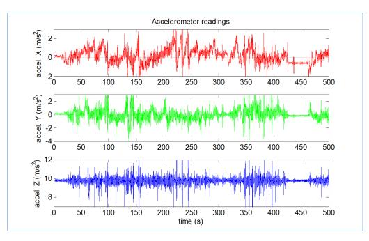
Figure 5.6: Sample accelerometer readings featuring two stops around t=[0;15] and t=[430;460] seconds. Bias combined with gravity effect makes the raw signal not adequate for detecting stops.
