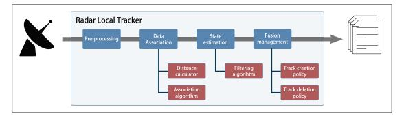
Figure 4.2: Selected processing scheme for the solution. Each sensor is processed individually, and local results are fused together by a global tracker.
