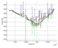
(c) Standard deviations of DGPS and GPS: East (upper blue bar) and North (lower green bar).
