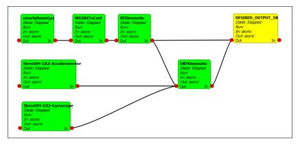
Figure 5.37: Sample fusion solution for getting vehicle position and linear speed
