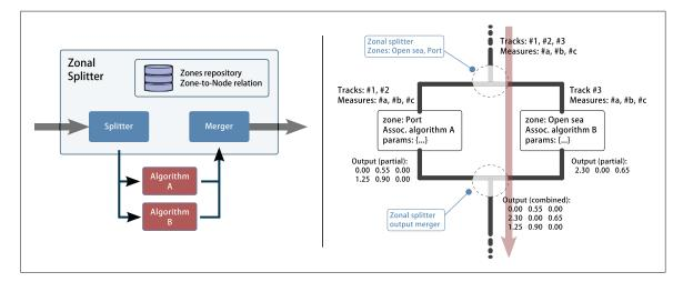
Figure 4.3: Zonal splitter processor divides input data in chunks (according to geographical location) that are processed using a different algorithm/configuration. Partial results are merged back to compose the output.
