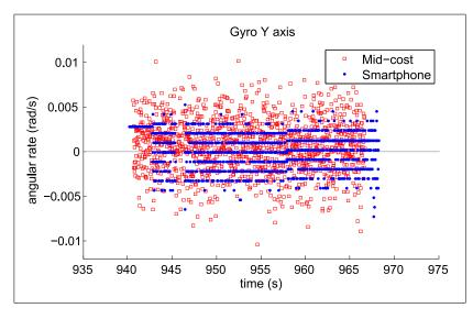
Figure 5.33: Gyroscope readings with the vehicle stopped.
