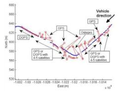
(b) DGPS and GPS solutions (red) and UKF filter solution (blue).
