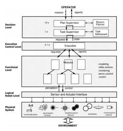
Figure 2.1: LAAS architecture for design and implementation of real time mobile robots
