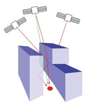
Figure 5.1: Urban canyon creates a degraded GPS environment where signals are blocked and reflected.
