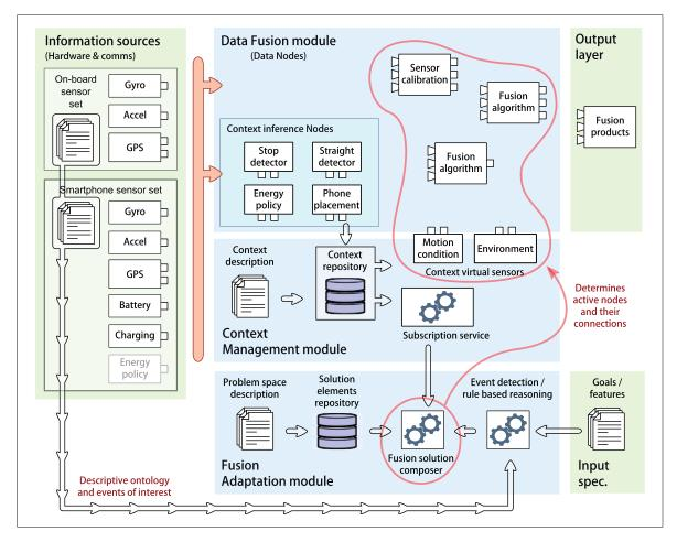
Figure 5.8: Instantiation of the designed adaptive navigation solution into the proposed framework
