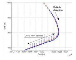
(b) Loss of accuracy in a soft urban environment (DGPS with 4 satellites) and UKF filter solution
