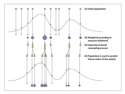
Figure A.4: Illustration of the sampling importance resampling process, inside the working cycle of a particle filter. Adapted from (Van der Merwe et al., 2000).
