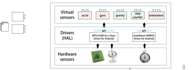
Figure 3.2: Virtual sensors abstraction in a smartphone equipped with Android OS. Step counter sensor can represent a real piece of hardware or a software process over accelerometer data
