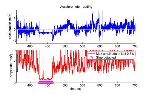
Figure 5.16: Sample accelerometer readings, processed signal, and output of the car stop detection module. This figure shows the validity of the applied strategy.
