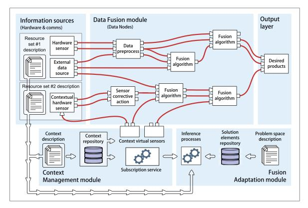
Figure 3.1: Architecture of the context-based adaptive sensor fusion system
