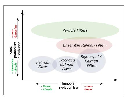
Figure A.1: Comparative chart of several filtering algorithms, considering two variables: how complex/powerful is the probability distribution used to described the estimated state of the system, and the expressiveness of the prediction model supported by the filter.
