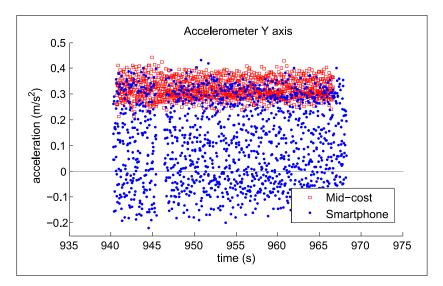
Figure 5.32: Accelerometer readings with the vehicle stopped. Note that bias is not corrected on these samples.
